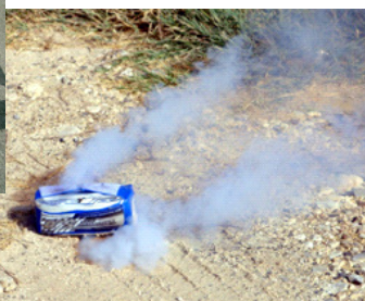
Pete Dubree "over-amped" a six cell pack. Outer wrapper burst (left). Pete decided to "neutralize" the pack by puncturing it with a long screwdriver. Smoke and fire started immediately. Lots and lots of very acrid smoke and fire. Not sure I'd try that. Battery later safe to transport for disposal.
