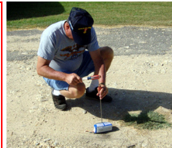
Pete Dubree "over-amped" a six cell pack. Outer wrapper burst (left). Pete decided to "neutralize" the pack by puncturing it with a long screwdriver. Smoke and fire started immediately. Lots and lots of very acrid smoke and fire. Not sure I'd try that. Battery later safe to transport for disposal.
